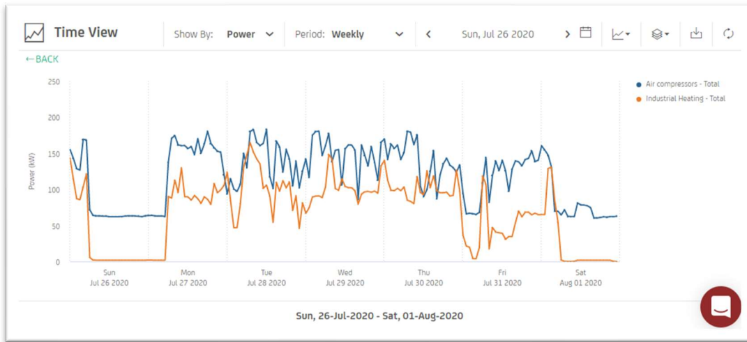
Figure 1: Compressed Air kW vs. Industrial Heating kW 2
