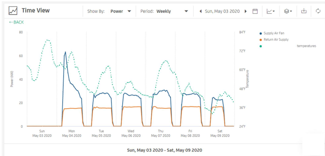
Figure 4: Final post period AHU fan kW
