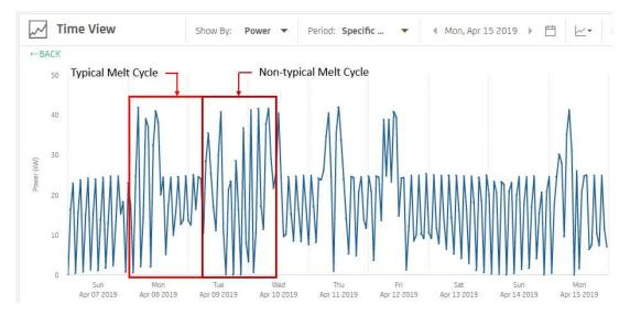
Site Watch Application – Daily and weekly reports showing furnace electricity input over time are used to track periods of excessive use. Time-view plots over 6-hour periods are used to indicate whether a furnace is operating in manual mode. Plant personnel can be notified of improper procedures and corrective action can be taken.
