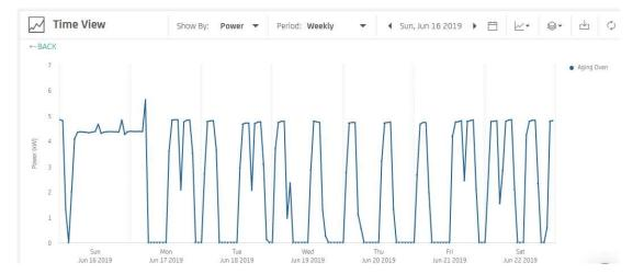
**Site Watch Application** – The Power Radar mobile app is used to access time-view of heat treatment furnaces, allowing the user to track when a treatment started, and ensuring proper equipment cycling through 3<sup>rd</sup> shift hours (nights and weekends).
